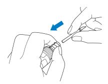
2 Twist on the holder cap to attach it to the holder.
