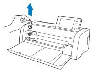
4 Use a commercially available brush to clean around the feed slot and the carriage.
