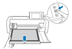
▶ The mat is fed in to complete the preparations for cutting.
