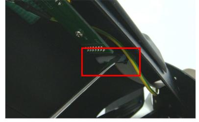
5. Pull out flat cable on control panel, and then remove the top cover.
