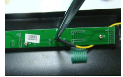
6. Use Phillips screwdriver to loose screw on control panel board.
