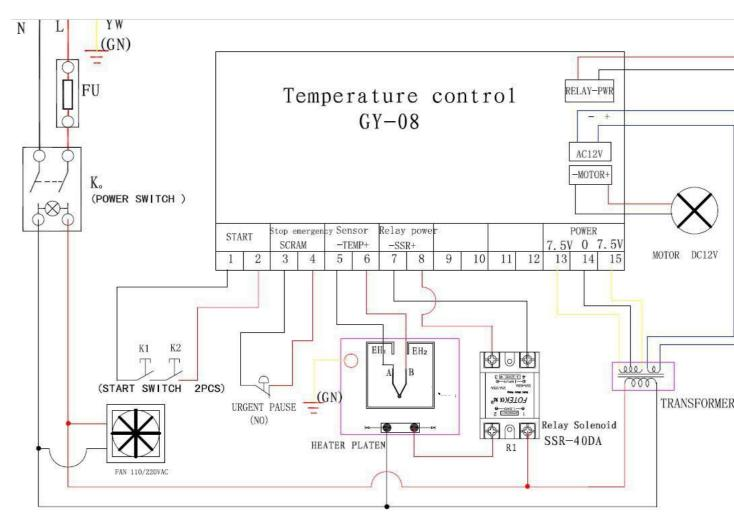
K.: Power Switch T: Bridge Transformer EH1 EH2: Heating Pipe
