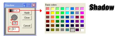
The "o" symbol represents the angle of the orientation of the shadow when compared to the image from which it originates. "D" represents the distance between the image and its shadow. When you are satisfied with the selected parameters, press on **Apply**.
