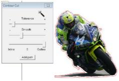
Use the magic wand and click to the left near the image, the vectorisation tool will create automatically an outline. Use the sliding cursor Tolerance to adjust your outline. Your outline contains too many segments, use the sliding button Smooth to remove segments and generate a smoother outline
