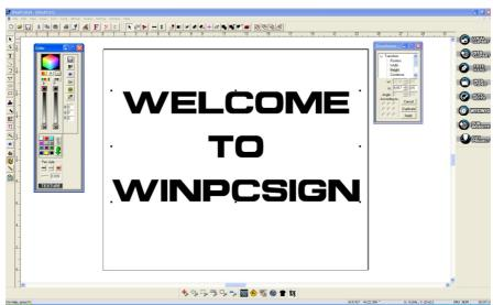
The "working screen" represents your page according to the selected dimension and orientation of your sign or the material putting on the plotter. You will also see the tools bar, the color palette, function bar and, on top of your screen and zoom bar at bottom of the screen
