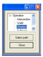
From Operation screen, selects **Welding/Shadow**, then click **Select path**. With the help of the mouse, click on the object that you want to create a shadow. WinPCSIGN will automatically open shadow configuration screen.
