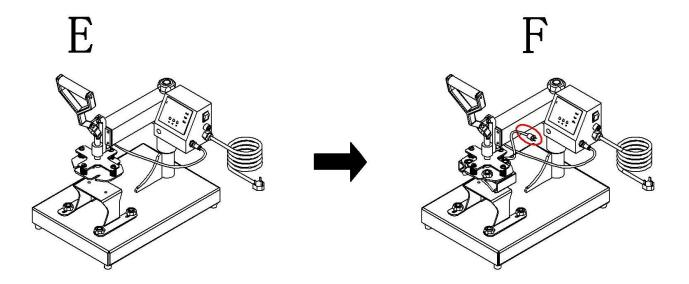
Tighten the screws of cap heat element, then connect the wire to the power connector.
