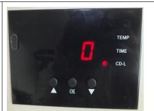
Press button after time setting; the display shows the temperature starts to rise. "CD-L" shows the time counting down during your transfer.
