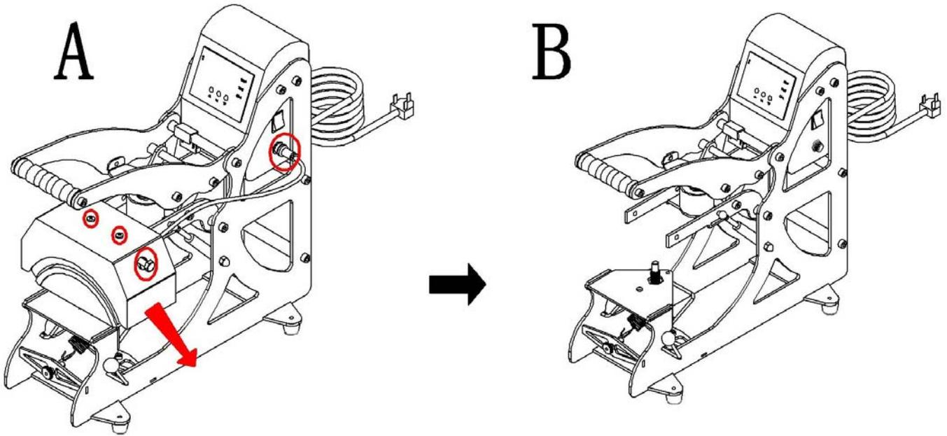
Remove the male socket which is connected to Female socket set in side of electrical case;
