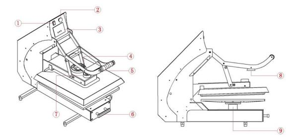
① Power Switch④ Pressure AdjusterØ Electromagnet
