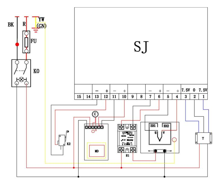
KO: Power Switch EH1 EH2: Heating Pipe T: Transformer K2: Limit Switch SJ: Thermostat R1: Relay FU: Fuse(16A/25V) C: Magnet MD : Magnet Driver
