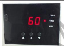
Press button after the temperature setting and the time light is ON. Press Up "△" or Down "▽" button to set time according to different transfer material.
