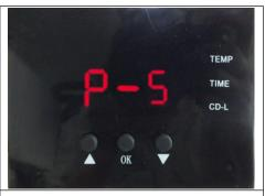
If there is a difference between the actual temperature and temperature shows on the controller, you can use **P5 mode** to calibrate the difference.
