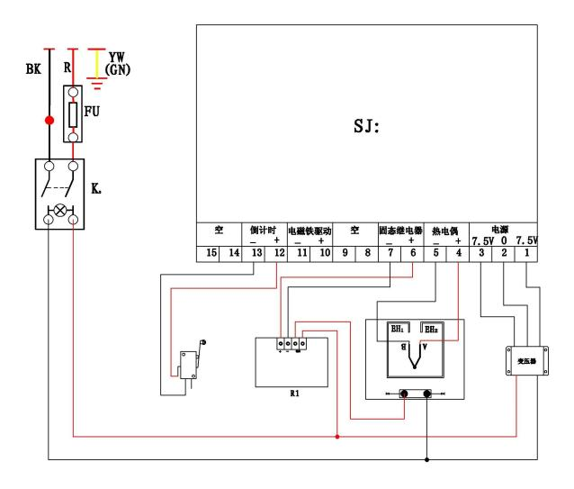
K<sub>0</sub>: Power Switch T: Transformer SJ: Digital Controller R1:Relay
