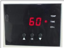
Press button after temperature setting and the time light is on. Select with arrows the time
