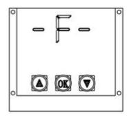
3. Press "OK" button to enter TEMPERATURE setting. When the TEMP indicator blinks, use Up/Down button to set the required temperature. (Temperature adjustable range: 100-225 C/212-437 F)
