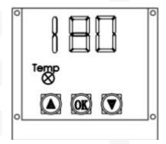
4. 4. Press "OK" button to enter TIME setting. When the TIME indicator blinks, use Up/Down button to set the required time. (Time adjustable range: 0-999S)
