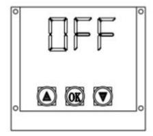
2. Press the "OK" button will shows the degrees Celsius "C". You could use the Up or Down button to switch between degrees Celsius and degrees Fahrenheit.
